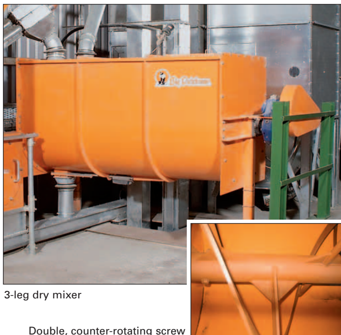
Double, counter-rotating screw
