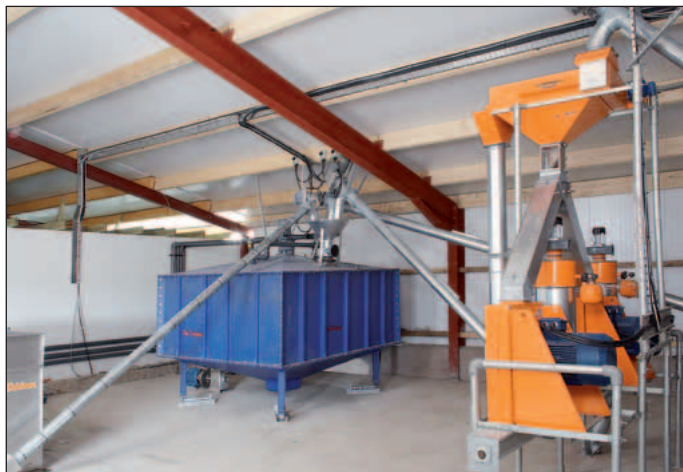
Double mill in combination with HYDROMIX liquid feeding system
