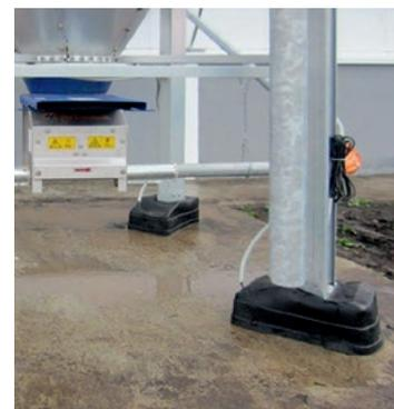
Cover for silo foot for secure weighing in extreme weather
